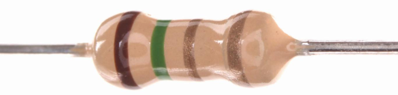
**Resistors** are measured by their resistance in *ohms*  $(\Omega)$ , often seen in *kilohms*  $(k\Omega)$
