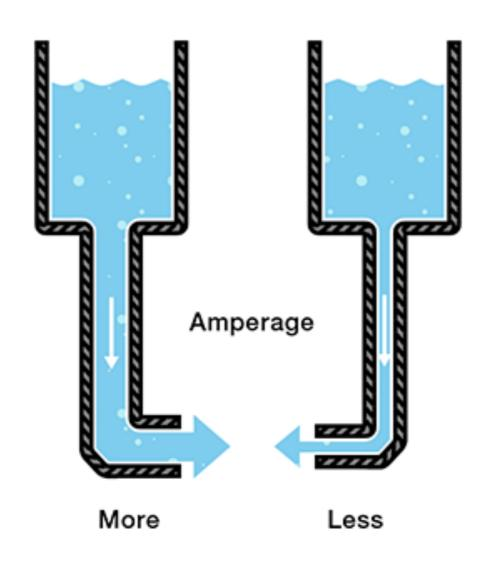
**Resistance** is a measure of a material's ability to oppose the flow of electricity. It is measured in *Ohms*.
