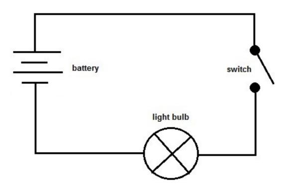
Every circuit has to have a **source** of electrical energy and a **load** that uses the energy.
