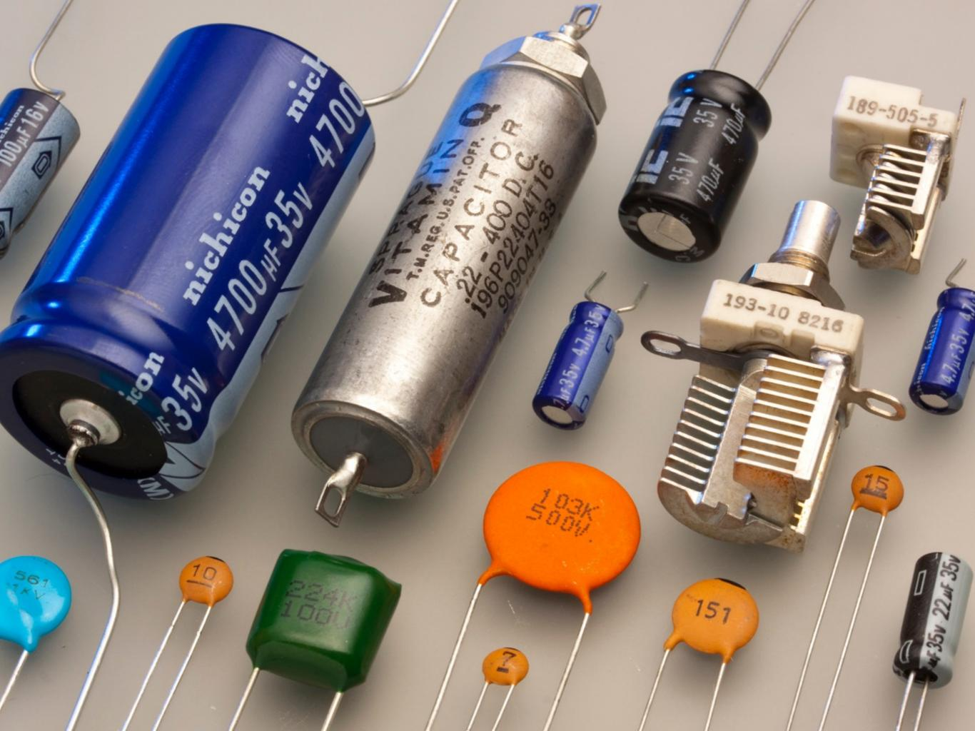
Sometimes they are **polarized**, meaning current can only flow through them in a specific direction, and sometimes they are not.
